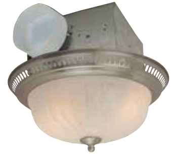
TFV70L-DSS - Decorative Vent Trim: 13.4" Dia x 6" H Housing: 5.6" D x 7.6" W x 8.6" H 70 CFM; 3.5 Sone; 2 - 60 Watt
