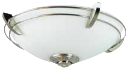
LK207-(FINISH)-LED - Light Kit 13.7"W x 4.5"H 2 - 9 Watt LED Bulbs Included 3000K Color Temp, 1500 Lumens, CRI 80 Glass: Opal Frost (BN, BNK), Amber Frost (OB) Finishes: BN, BNK, OB
