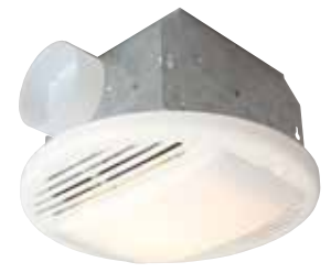
TFV50L - Builder Series Vent Trim: 12.3" Dia x 2" H Housing: 5.6" D x 7.6" W x 8.6" H 50 CFM; 3.5 Sone; 1 - 60 Watt
